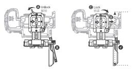
When using the LCD screen protection bracket, the maximum width compatible with the V-mount battery is 80mm / 3.1in.
