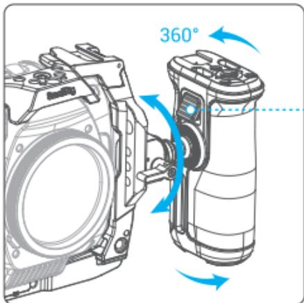
Step 2: Push the button to enable 360° bi-directional rotation for seamless operation.
