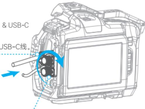
Step 3: Tighten the thumbscrews to secure the cable.
